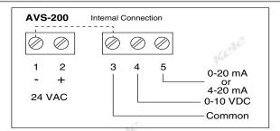
Note: Any device sharing a transformer with the AVS-200 must have a common power negative "-" and signal negative "-" terminal, and polarity must be observed. Otherwise, a separate transformer must be used.
